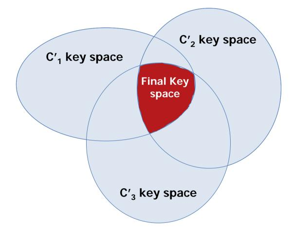
Multiplying the number of faulty ciphertext directly reduces the final key space size and therefore the complexity of the exhaustive search
