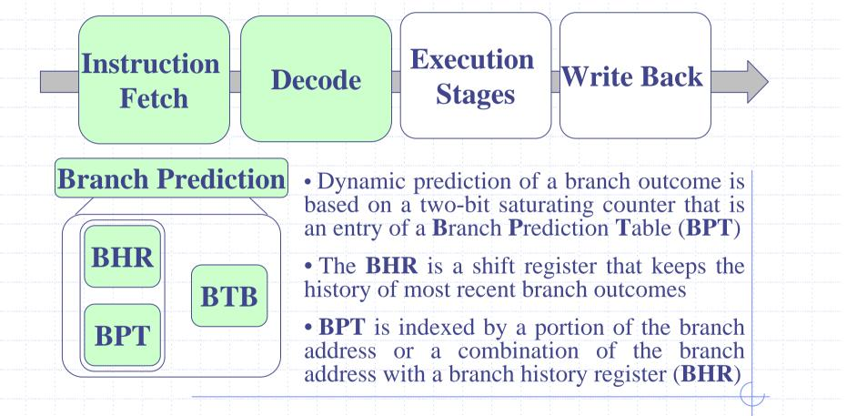
Branch Target Buffer (BTB) is a cache structure indexed by the low order part of the branch address; the cache data is the last target address of that branch
