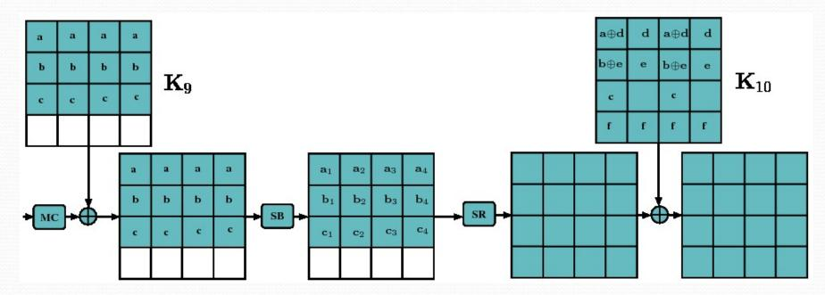
Requires two faulty ciphertexts (each with 3 simultaneous byte faults) to retrieve 12 bytes of the AES 10<sup>th</sup> round key.
