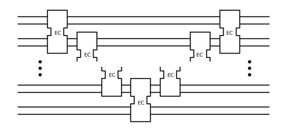
SCA Resistant Circuit Manchester Encoding 0 = (0,1) 1 = (1,0)Gadgets Encoding and Error Cascading propagates invalid 00
