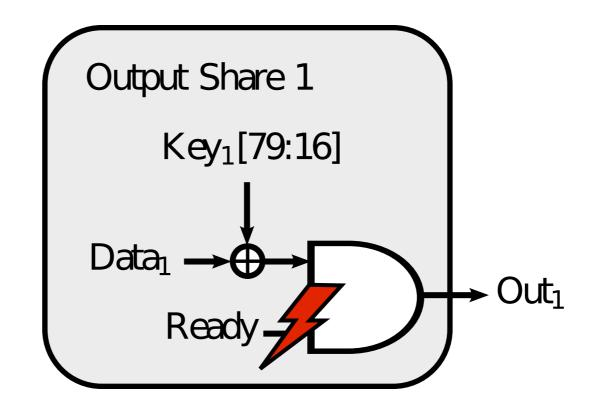
Fault on ready signal can reveal all intermediate results
